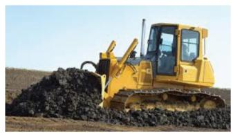
A bulldozer is a crawler (continuous tracked tractor) equipped with a metal plate known as a blade used to push large quantities of soil, sand, rubble or other materials during construction. Bulldozers are often large and powerful. Bulldozers are often used in road building, construction, mining, forestry, land clearing and any other projects requiring highly mobile, powerful and stable earth-moving equipment.
